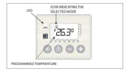
There is an LED light on the control panel: when the system is in heating mode and the room temperature has not yet reached the desired temperature programmed by the user, the LED is RED. Once the room reaches the programmed temperature, the LED turns GREEN.
