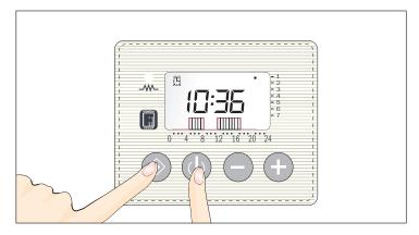
A dot will blink on the screen next to the days of the week. The current day can be selected using the plus or minus key. Use the 'mode' key to confirm the selection. The number corresponding to the hour will blink. Set the correct time using the plus and minus keys. Confirm the selection with the 'mode' key. The number corresponding to the minutes will blink. Set the correct minutes using the plus and minus keys. Confirm the selection with the 'mode' key
