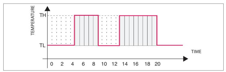
TH is the desired ambient temperature during the time periods selected; TL is the (reduced) desired temperature outside the selected time periods.
