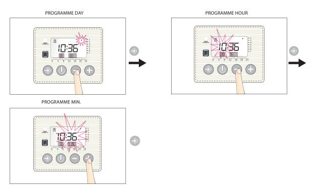
You can now assign a setting to each day of the week. When a segment appears between two times on the programming bar (at the bottom of the screen), this indicates that the TH temperature level has been selected for this period. The absence of a segment indicates that during this period, the radiator will keep the temperature at the TL level.
