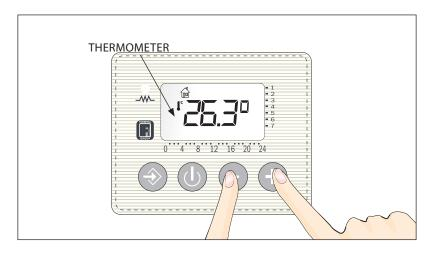
Press the 'stand-by' and 'mode' keys at the same time and hold for three seconds.
