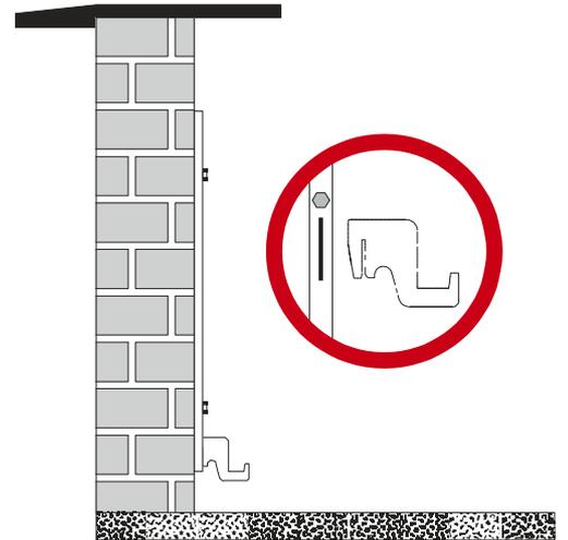
5. Stand the Economiser Radiator vertically in front of the vertical mounting bars and remove the top ventilation grille. Next, lift the radiator and position over the hooks so that each hook locates into a rib.
