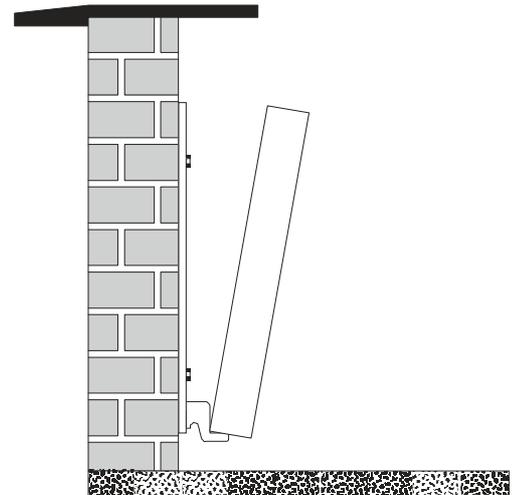
6. To fit the upper hooks, tilt the Economiser Radiator Slightly towards you and locate the hooks into the Upper section of the vertical mounting bars. Slowly Set the radiator upright while lifting the hooks upwards, Then lower them into the upper ribs of the radiator. Finally, replace the ventilation grille.
