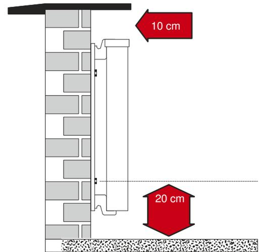
2. Mark the first and lowest drill hole location at a distance of 20cm from the floor and adjust the mounting bar using a spirit level to ensure that it is vertical before marking drill point for the upper bolt. Drill drive holes using 8mm masonry bit, fit screw anchor and tighten hexagonal bolt until bar is secure.
