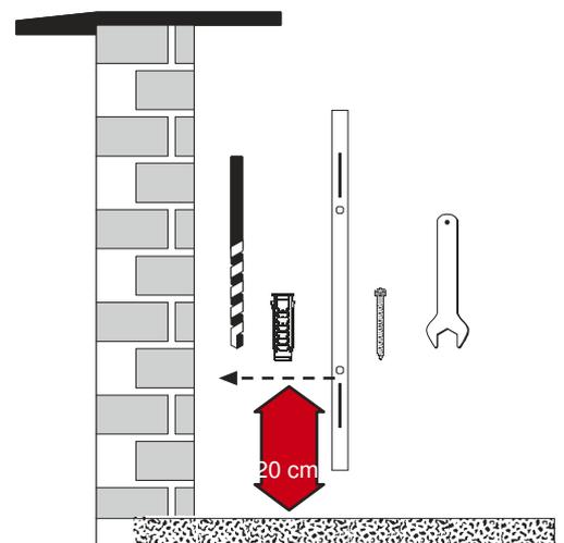
3. To locate position for second mounting bar, measure the length of the radiator, then count 3 x full ridges inwards from outer end panels. Note; although weight should be supported as evenly as possible, precise measurement is not required as radiator can be hung from a number of points.
