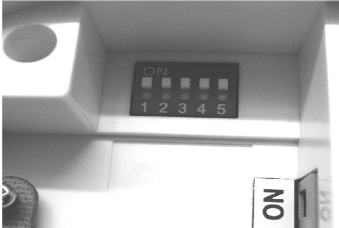
Disconnect AC power to the receiver unit and remove batteries from the programmable thermostat before attempting any adjustments of the RF address code switches and jumpers. If you are not sure how to carry out this procedure correctly, please contact a qualified electrician or heating engineer.
